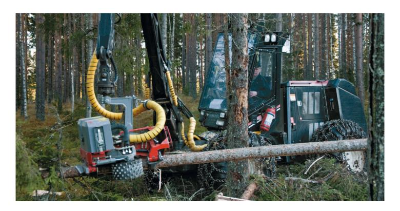
The Log Max 928 features a hydraulically driven saw with pressure controlled sawing force and flow controlled chain speed.
